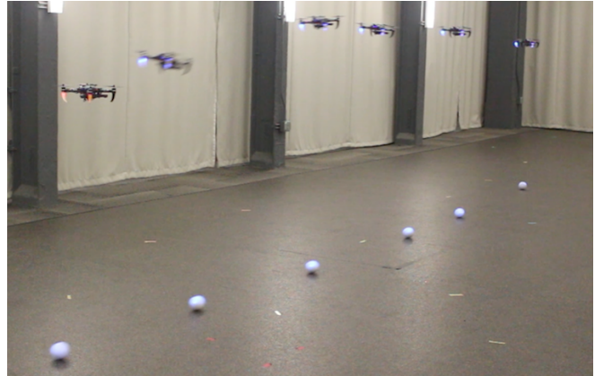
Fig. 1. A quadrotor accelerates to track a target moving at 1.5 m/s. The motion is planned in real time and considers the estimated trajectory of the target, the dynamics of the robot, the actuator limitations, and the camera’s field of view. All sensing and computation occurs onboard the robot and leverages only one downward-facing camera and an onboard inertial measurement unit.
